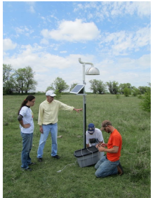
Fig. 6. New Mexico Tech solar-powered slow antenna installation. Battery box is being installed by Ron Thomas and Mason Quick, while being well-managed by our illustrious Brazilian team.
