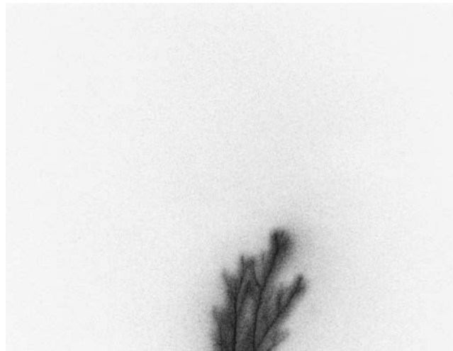
Fig. 16. The visible image taken by a 4 Picos camera aimed at the center of the aerosol cloud at a height of 80-120 cm above the plane, where the ball from which the discharge started is located. The camera was started by the current pulse with the ball going through the shunt 800 ns after the initial corona flare. Exposure time is 200 ns.
