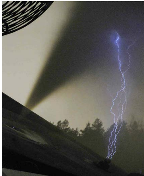
Fig. 2. Integrated photograph of discharges with 5-s exposure. Four upward positive discharges from the ball, which is connected through the shunt to the oscilloscope.
