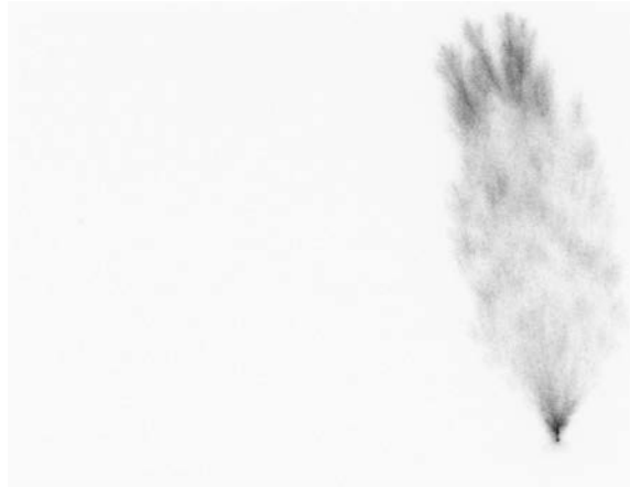
Fig. 15. The visible image taken by a 4 Picos camera, which includes both the starting leader a few centimeters long, with the streamer corona rising from the leader, and much less bright plasma structures on the top of the streamer corona, which can be stalkers . The camera was started by the current pulse from the ball going through the shunt 400 ns after the initial corona flare. Exposure time is 200 ns.
