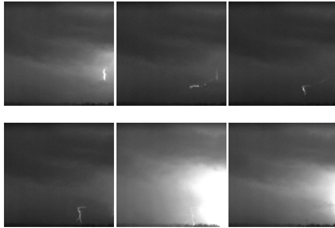
Figure 3 Optical images of leader and first return stroke processes the lightning from -4 ms to 1 ms. The time interval between the adjacent frames is 1 ms.
