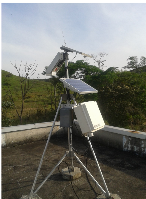
Figure 10 – Campbell Scientific CS110 EFM assembled on a metal tripod (JCR site)
