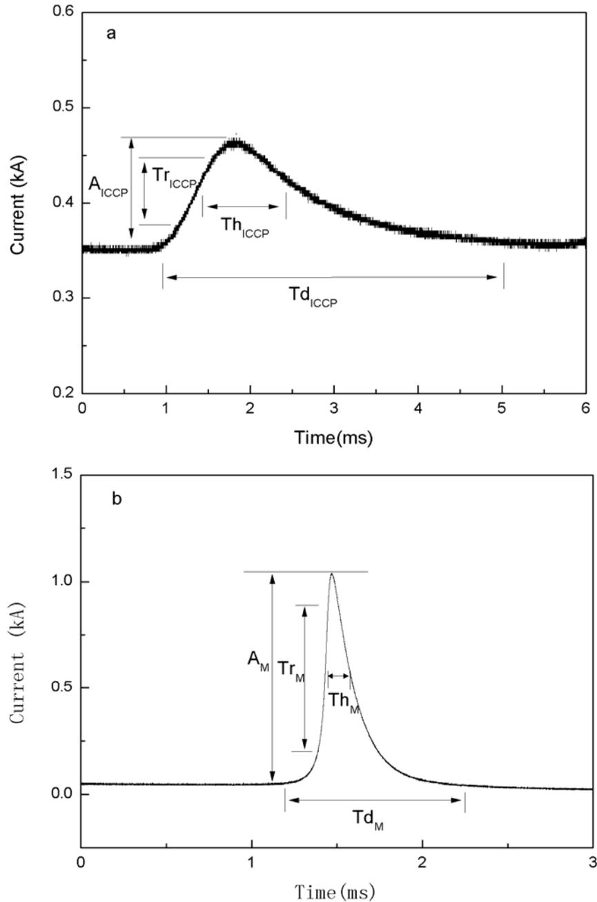
Figure 2 Current waveforms: a, initial continuous current pulse (ICCP) in triggered lightning T201102; b, M-component in triggered lightning T201107
