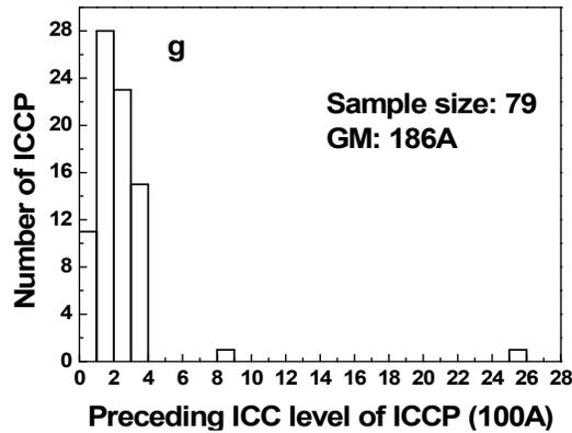
Figure 3 Distributions of characteristic parameters of initial continuous current pulse (ICCP) in triggered lightning: a, magnitude; b, charge transfer; c, duration; d, rise time from 10% to 90% peak; e, half peak width; f, interpulse interval; g, preceding ICC level
