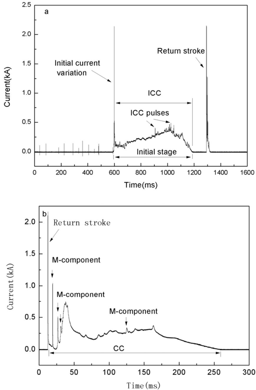
Figure 1 Current waveforms: a, initial continuous current (ICC) in triggered lightning T201102; b, continuing current (CC) in triggered lightning T201107
