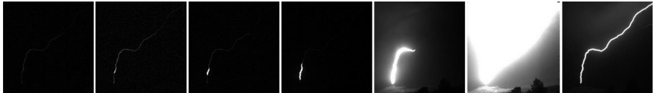
Figure 10 – A different M-component initiated by a bidirectional RL starting close to the tower T1 tip.
