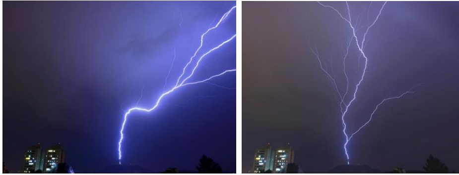
Figure 3 – Nikon D800 digital still images of UP1 (on left) and of UP2 (on right). Camera settings were as follows: ISO, 100; aperture, f/8; focal length, 20 mm; exposure time, 18.2 s.
