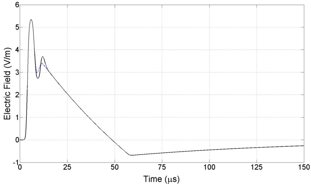
Figure 6. The MTL-model-computed return stroke electric fields with (black solid line) and without (blue dashed line) reflection at the bottom end of the branch. All parameters are the same as those used to compute the solid black line curve in Figure 3a. Reflection at the branch-end causes an increase in the amplitude of the secondary peak in the return stroke waveform. The time-window shown is 150  $\mu\text{s}$ .
