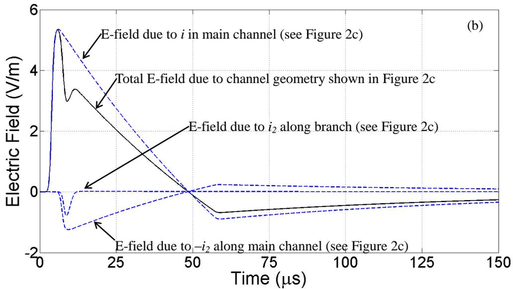
Figure 3. (b) The solid line shows the same waveform as in Figure 3a but additionally showing the contributions to the total electric field (waveforms shown with dashed lines) from the individual current components shown in Figure 2c.
