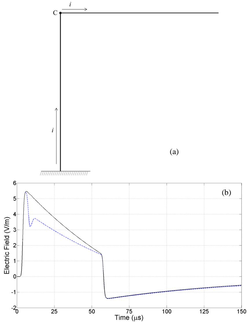
Figure 7. (a) The channel geometry including a long horizontal section attached at the upper end of a vertical return stroke channel. (b) The MTL model-computed return stroke electric field at a distance of 200 km for the geometry shown in (a) (solid line), and for the geometry including both the horizontal channel section and a branch connected at 500 m (see Figure 2) (dashed line). The time-window shown is 150  $\mu\text{s}$ .
