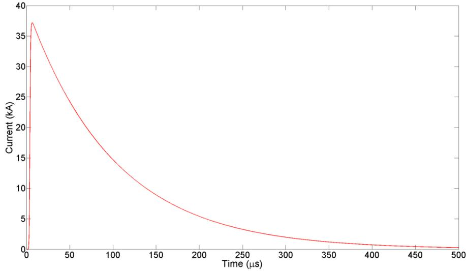
Figure 1. The incident return stroke current waveform computed using the Heidler function that is used in this study shown on a 500  $\mu$ s timescale. The current peak is about 37 kA and the zero-to-peak risetime is 6.6  $\mu$ s. The half-peak width is 72  $\mu$ s. This current waveform is representative of negative first return strokes.
