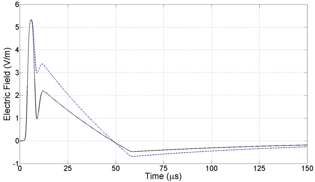
Figure 4. The MTL model-computed return stroke electric field at a distance of 200 km for the channel geometry shown in Figure 2c and the same parameters as those used to compute the solid line curve in Figure 3a, but with  $i_2/i_1 = 0.5$  (solid line). The electric field waveform for  $i_1/i_2 = 0.25$  (same as in Figure 3a) is also shown (dashed line) for comparison. The time-window shown is 150  $\mu\text{s}$ .
