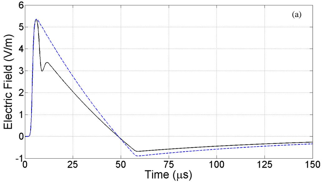
Figure 3. (a) The MTL-model-computed return stroke electric field at a distance of 200 km for a straight vertical channel with no branching (blue dashed line) and for the channel geometry shown in Figure 2c (black solid line) shown on a 150  $\mu\text{s}$  timescale. The presence of branch served to slightly decrease the magnitude of the opposite polarity overshoot.
