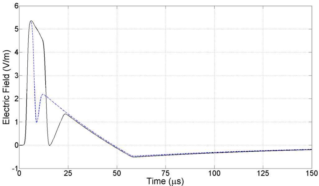
Figure 5. The MTL model-computed return stroke electric field at a distance of 200 km for the same parameters as in Figure 4, but with  $h_b = 1400$  m above the ground surface and the length of the ungrounded branch  $l_b = 1350$  m (solid line). Also shown is the electric field waveform for  $h_b = 500$  m (dashed line) for comparison. The time-window shown is 150  $\mu\text{s}$ .
