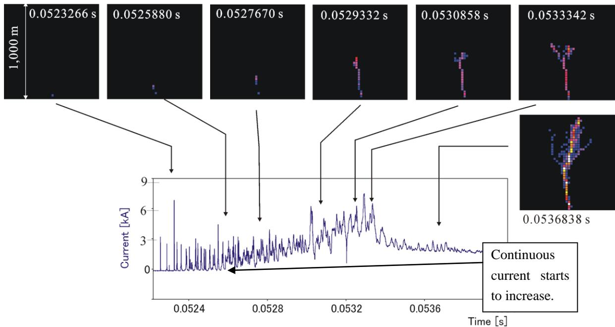
Figure 9 Negative upward leader and corresponding current waveform.
