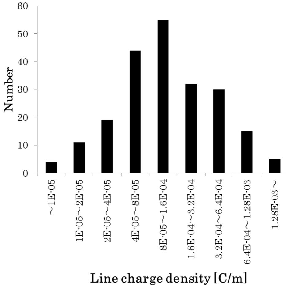
Figure 13 Histogram showing the line charge density of the extended leader segment produced by step propagation.
