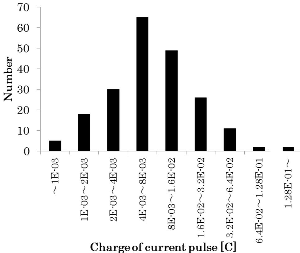
Figure 12 Histogram of the charges of the current pulse in positive upward lightning.
