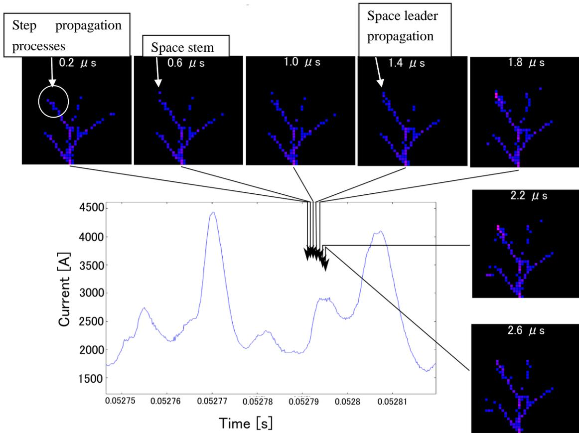
Figure 11 Stem and space leader of negative upward leader with the current pulse
