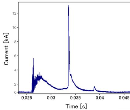
Figure 3 Entire current waveform of positive upward lightning.
