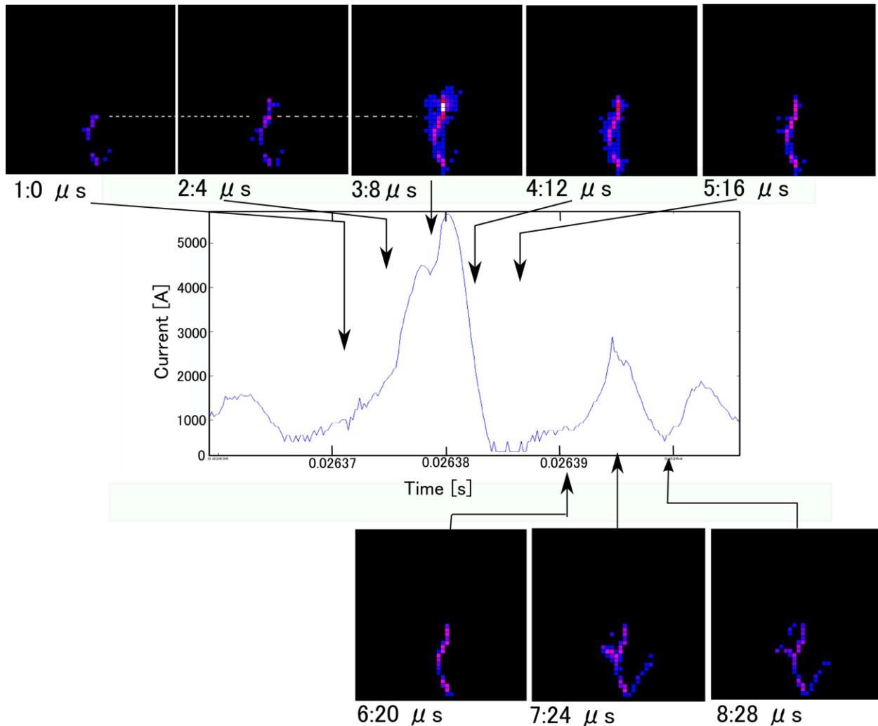
Figure 5 Step formation of upward leader and the corresponding current pulse.
