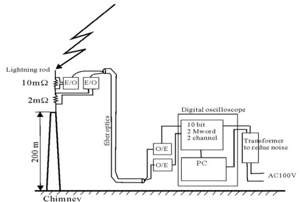
Figure 2 Current measurement system.
