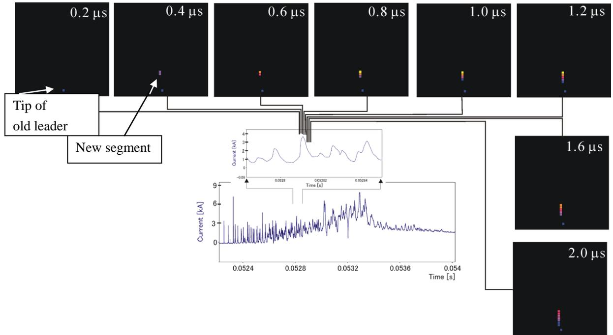
Figure 10 Step formation of negative upward leader and corresponding current waveform
