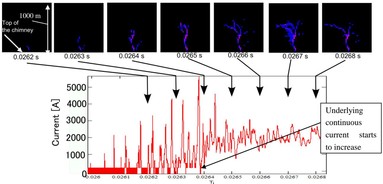
Figure 4 Negative upward leader and corresponding current waveform.
