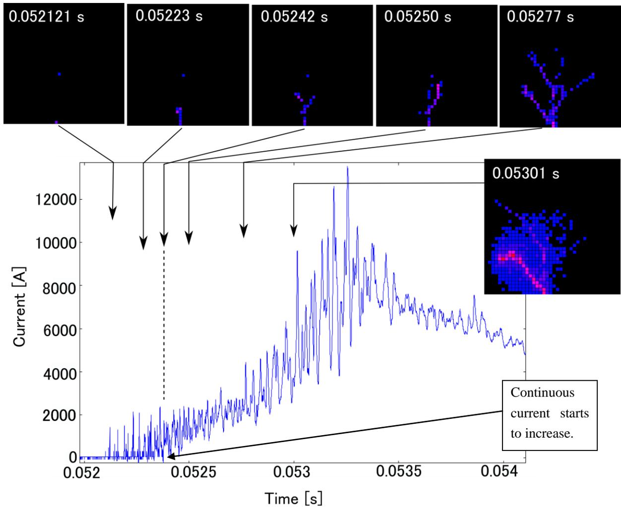
Figure 8 ALPS images showing upward negative leader and the corresponded current waveform
