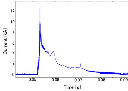
Figure 7 Current waveform of positive upward lightning
