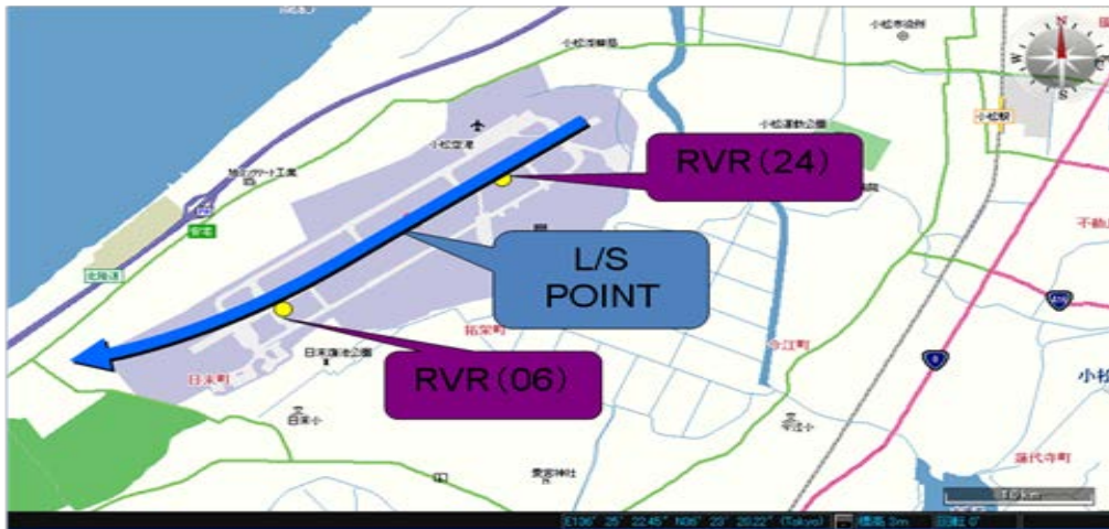
Figure 5 Map of Komatsu Airport, runway directions are NE, 060 degrees and SW, 240 degrees, respectively.
