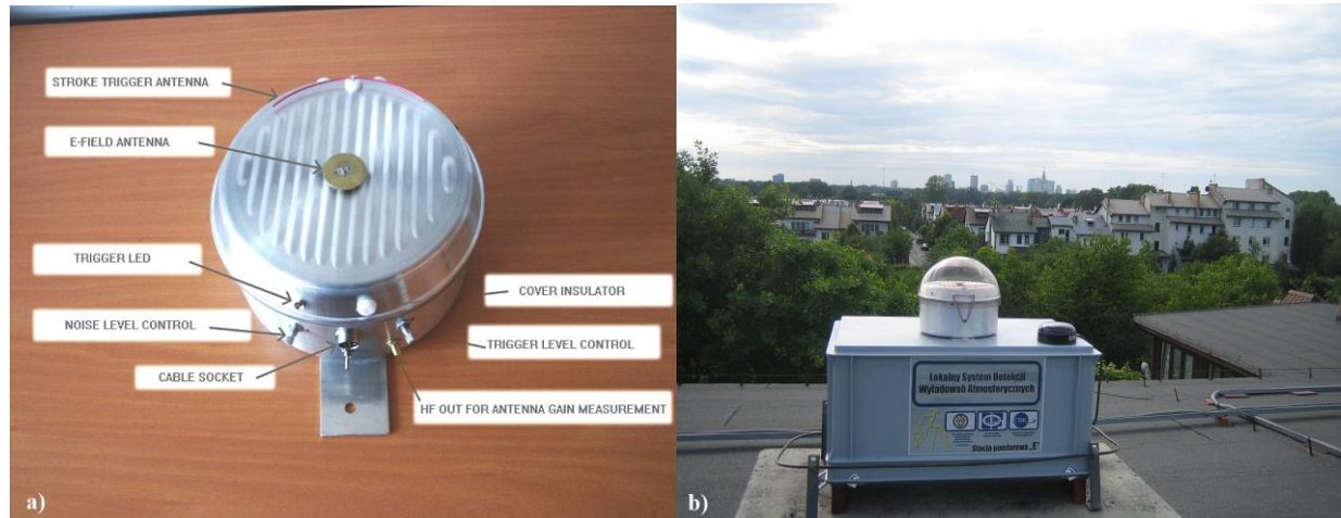
Figure 1. One of six E-field antennae devices used by the LLDN in Warsaw region (panel a) and general view of measuring station E located on the roof of Space Research Centre building (panel b).
