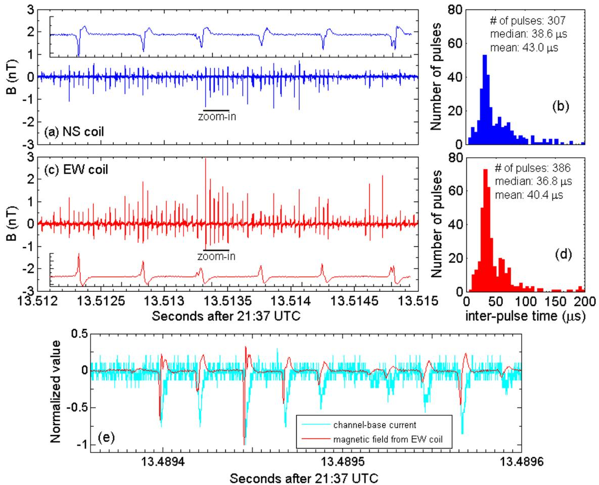
**Figure 2.** Panels (a)-(d): The LF magnetic field over 3 ms showing the periodic pattern of small in-cloud discharges. The statistics of more than 300 pulses (with magnitude five times the noise level) scattering over 25 ms indicates that the inter-pulse intervals are typically 20-45  $\mu\text{s}$ . Panel (e) compares the channel-base current waveform and the magnetic field
