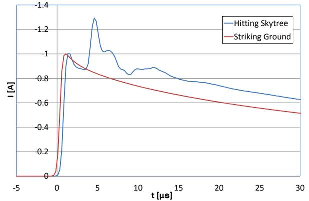
Fig. 4 Calculated current waveforms of subsequent return strokes hitting 634-m tower or ground by using an electromagnetic model of return stroke.
