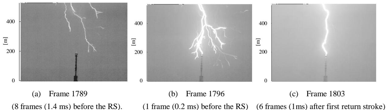
Fig. 7 Upward connecting leader and return stroke imaged by high-speed camera (Flash 2013-7)
