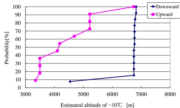
Fig. 2 Difference of cumulative frequencies of  $-10^{\circ}\text{C}$  altitude depending on the type of flashes when they hit the tower.
