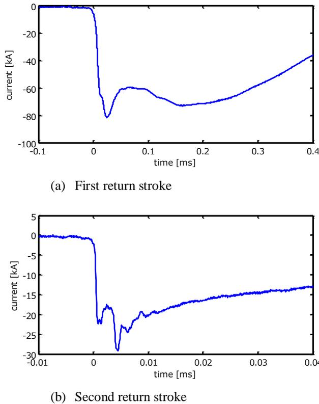
Fig. 3 Current waveforms of return strokes in negative downward flash (Flash 2013-7).
