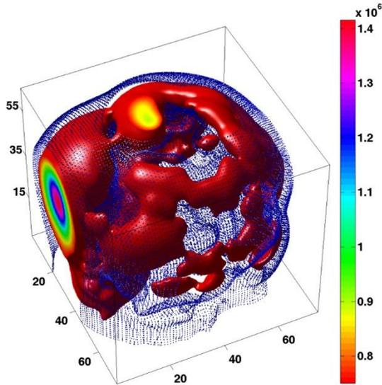
Fig.3. Spatial structure of the total electric field. The red surface corresponds to the electric field magnitude  $7.5 \text{ kV/cm}$ . The surface represented by the blue cones corresponds to the electric field magnitude  $7 \text{ kV/cm}$ . The plane  $z=0$  corresponds to the ground level, the colour scale is graduated in  $\text{kV/cm}$ , the horizontal and vertical axes are graduated in decimetres.
