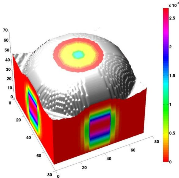
Fig.1. Distribution of the steady-state component of the electric charge density in the vicinity of the artificial aerosol cloud. The colour scale is graduated in  $\text{C/m}^3$ , horizontal and vertical axes are graduated in decimetres.
