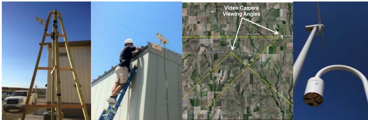
Fig. 2. (From left to right) Video camera installation at the Operations & Maintenance Building; video camera installation at the sub-station; map of the video camera viewing angles; view of an electric field mill installed at the wind farm.
