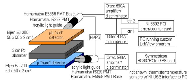
Figure 2: Diagram of the ground-based cosmic ray muon detector.
