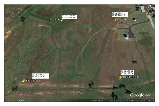
Figure 3: Image of the four cosmic ray muon detector array developed in Norman, OK [Google 2014].
