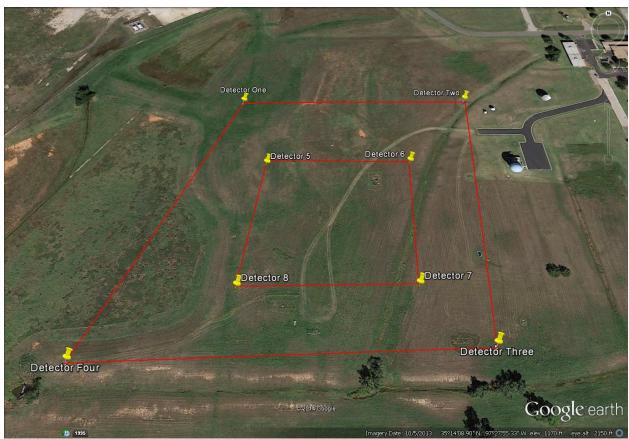
Figure 8: An image of a proposed expansion of the ground-based cosmic ray muon detector array. This expansion adds four additional detectors arranged in a ~100 m square in the center of the existing array [Google 2014].
