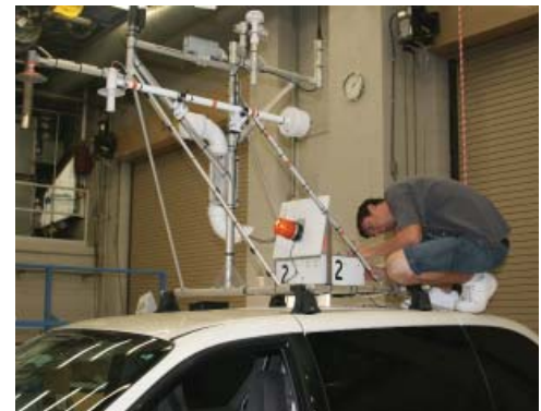
Mobile mesonets with roof-mounted instruments transmit real-time temperature, humidity, pressure, wind speed, wind direction, vehicle orientation and GPS location to a central command vehicle.
