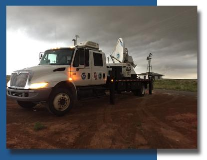
NSSL's NOXP is a dual-polarized X-Band mobile radar, and is more sensitive to smaller particles than NEXRAD's C-Band radars. It is capable of detecting tiny water droplets or snowflakes. This mobile radar can be driven into position as a storm is developing to rapidly scan the atmosphere at low levels, below the beam of WSR-88D radars. NSSL has used mobile radars to study tornadoes, landfalling hurricanes, dust storms, winter storms, mountain rainfall, and even swarms of bats.
