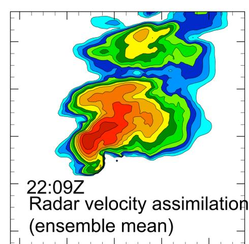
Analyses produce a supercell storm with low-level rotation. Less detailed than is possible with radar data, but shows promise in radar data-poor areas (e.g., mountains, off-shore)
