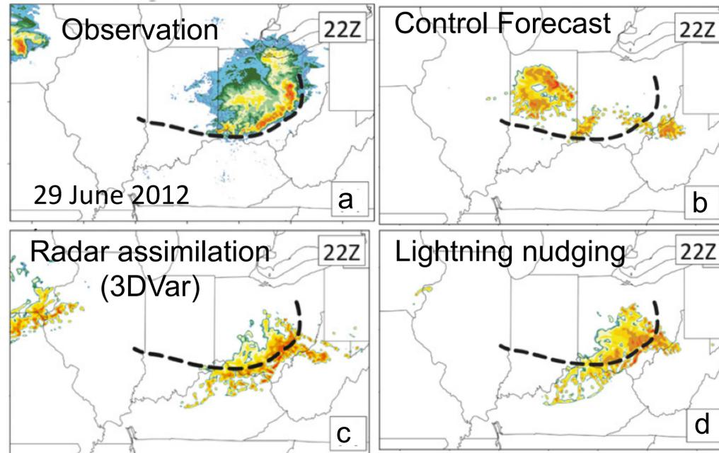
6-hr forecasts of radar reflectivity of a severe wind storm (derecho) with lightning nudging (ENTLN) or cycled radar 3DVAR methods.
