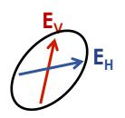
Beam is elliptical in shape and H is not parallel to the surface of the earth
