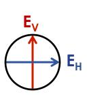
Beam is circular in shape and H is parallel to the surface of the earth
