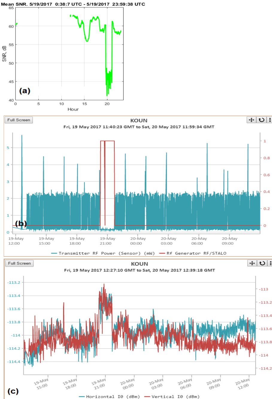
Fig.6. (a): SNR from ground clutter collected with KOUN 19 May 2017 using VCP-52. (b) ROCSTAR data on the transmitter power. (c) Same as in (b) but for noise levels in the horizontal (blue) and vertical (brown) channels.
