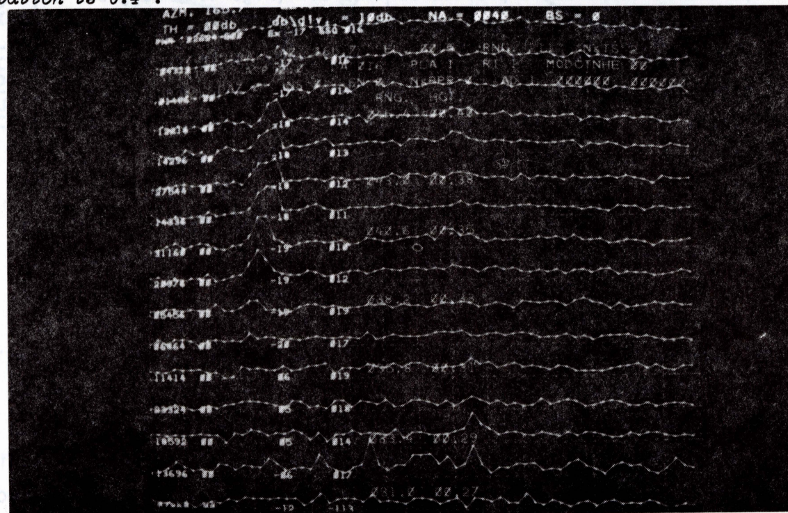
Figure 4.4.--Consecutive spectra collected at 0935 CST (see Fig. 4.3). The azimuth is 165.7^\circ , the vertical scale is 10 dB/div, and distance to first range gate is 31 km.
