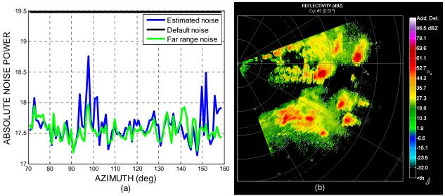
Fig. 4 (a) Noise estimates compared to the default and the far range noise, and (b) reflectivity field with additional detections obtained using estimated noise highlighted in white.
