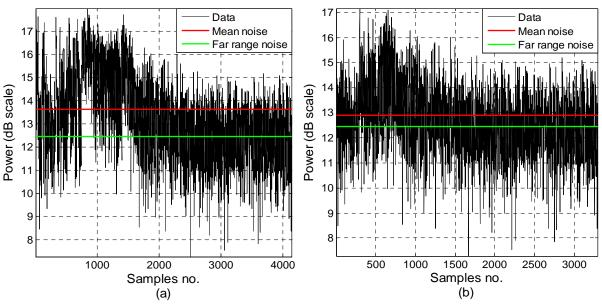
Fig. 2 (a) Power range profile after the first two steps of the algorithm.(b) Range power profile obtained after the step that applies the profile filter which discards 10 or more consecutive powers larger than the median.
