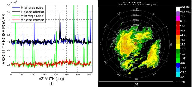
Fig. 5 (a) Noise estimates compared to the far range noise, and (b) noise estimates from the long and the short PRT.
