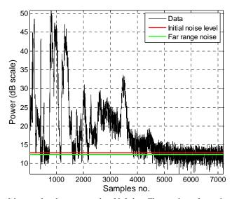
Fig. 1 Power range profile of data at the elevation angle of 0.5 deg. The number of samples at each range bin is 15 and the radar return is oversampled by 4.
