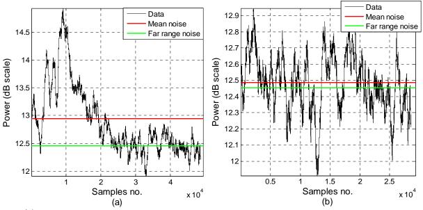
Fig. 3 (a) Range power profile obtained after applying the profile filter, and performing the running average of 750 points. (b) Range power profile obtained after applying twice the running average filter.
