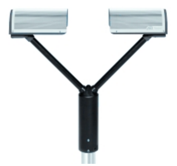
Above: Unmodified PARSIVEL 2 laser distrometer
