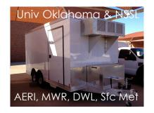
Collaborative Lower Atmospheric Mobile Profiling System (CLAMPS) (under construction)
