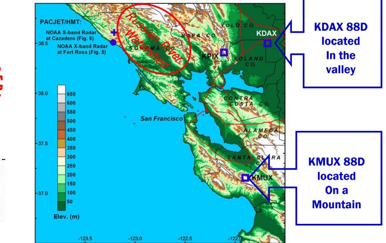
Poor WSR-88D coverage over Russian River watershed (88D radars are either blocked by terrain or overshooting the tops of the terrain-induced precipitation). NWS and KPIX worked together to find an optimal site for the TV radar.
