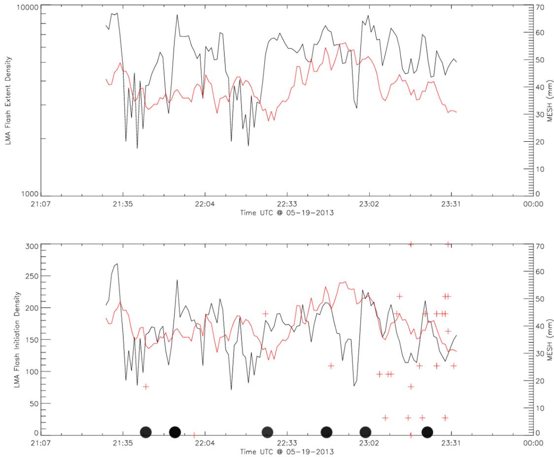
Fig. 11. Top: Time-series of Flash Extent Density (black) and MESH (red) values. Right: Time-series of flash rate based on flash initiation density (black), MESH (red) values, SHAVE reports marked with plus signs indicating hail size (in mm) and time, and black circles along time axis indicating time of 2sigma lightning jumps (2145, 2155, 2227, 2247, 2301, and 2323 UTC).
