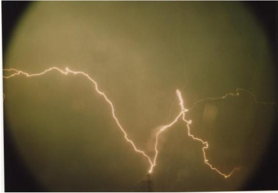
Figure 6 Still image of positive upward lightning
