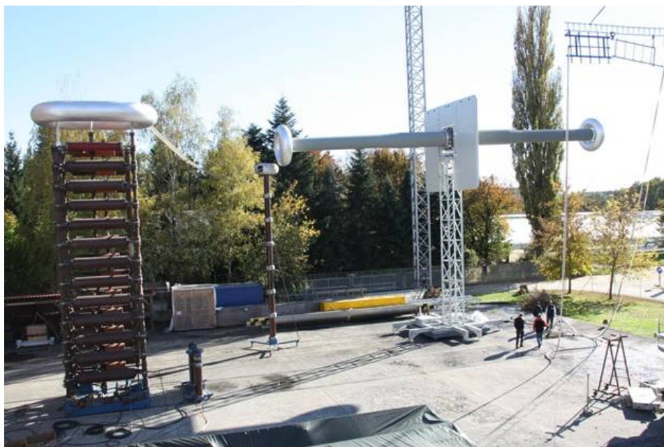
Photo 11: Switching impulse test of wallbushing, Graz University of Technology
