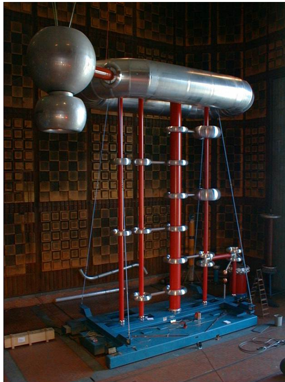
Photo 5: New 1500 kV DC generator in test position, Graz University of Technology
