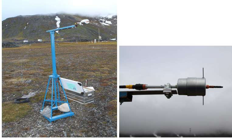
Figure 1: Left: The atmospheric electricity station. Equipment for measuring, recording and transmission of the vertical component of electric field E_z . Right: Rotating-dipole sensor for E_z measurements.
