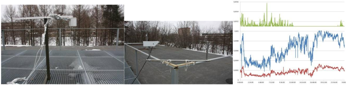
Figure 1. Exterior view of devices (EFS-2/50 (left) and RIO) and an example of recording data.
