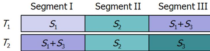
Fig. 4.5. Depiction of possible overlaid echo occurrences in the SPRT algorithm.
