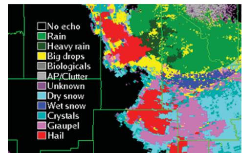
Dual-polarization technology, when added to the WSR-88D radar network, will help forecasters identify different types of precipitation within radar data.
