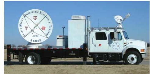
One of the mobile 5-cm SMART-Rs was recently modified to perform simultaneous transmit/receive dual-polarization measurements. As a research radar, the SMART-R can transmit real-time data products back to the Hazardous Weather Testbed in Norman, OK, where researchers and forecasters are testing new techniques.
