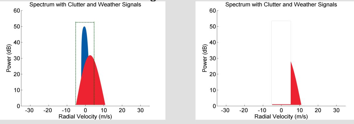
Clutter filtering is also difficult when collecting a small number of  $\bullet$ pulses (e.g., detection scans, beam multiplexing), techniques that could be useful on a phased array
