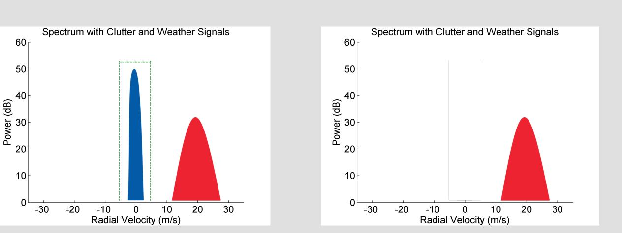
When the weather velocity is near zero, clutter filtering can affect • the estimates of meteorological variables.
