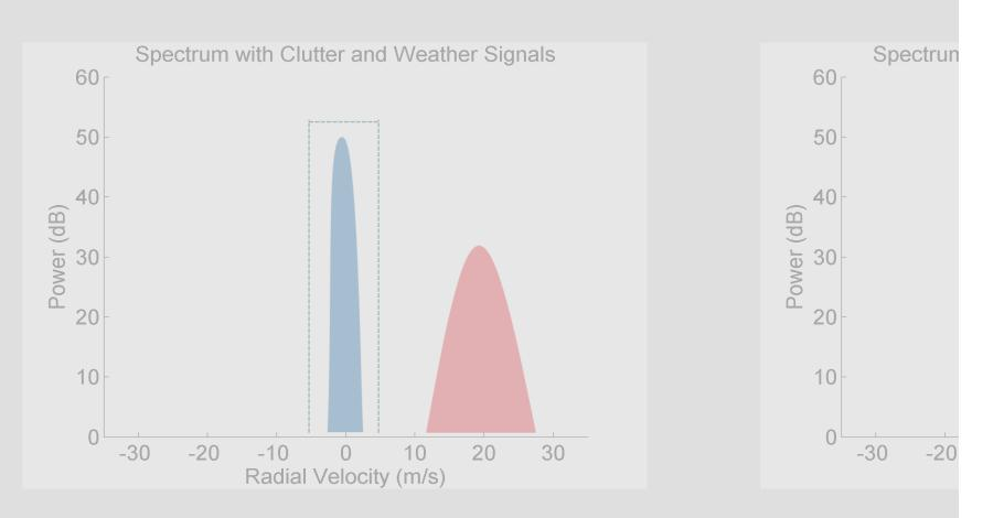
When the weather velocity is near zero, clut the estimates of meteorological variables.
