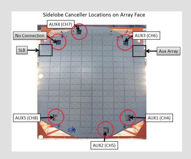
Combining multiple channels from antennas at different positions allows spatial filtering.
